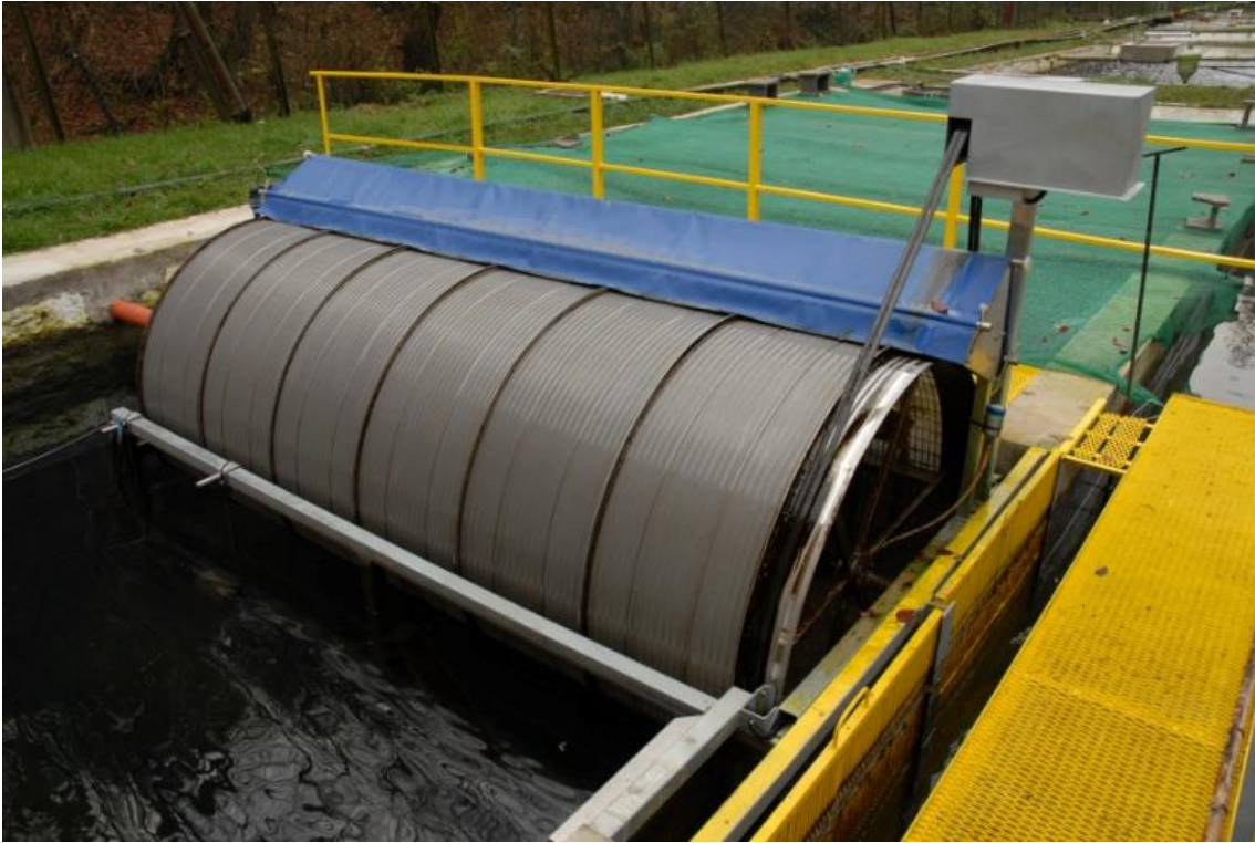
Figure 6 – Drum filter in the open air RAS of the Hoits and Rieger intensive trout farm
