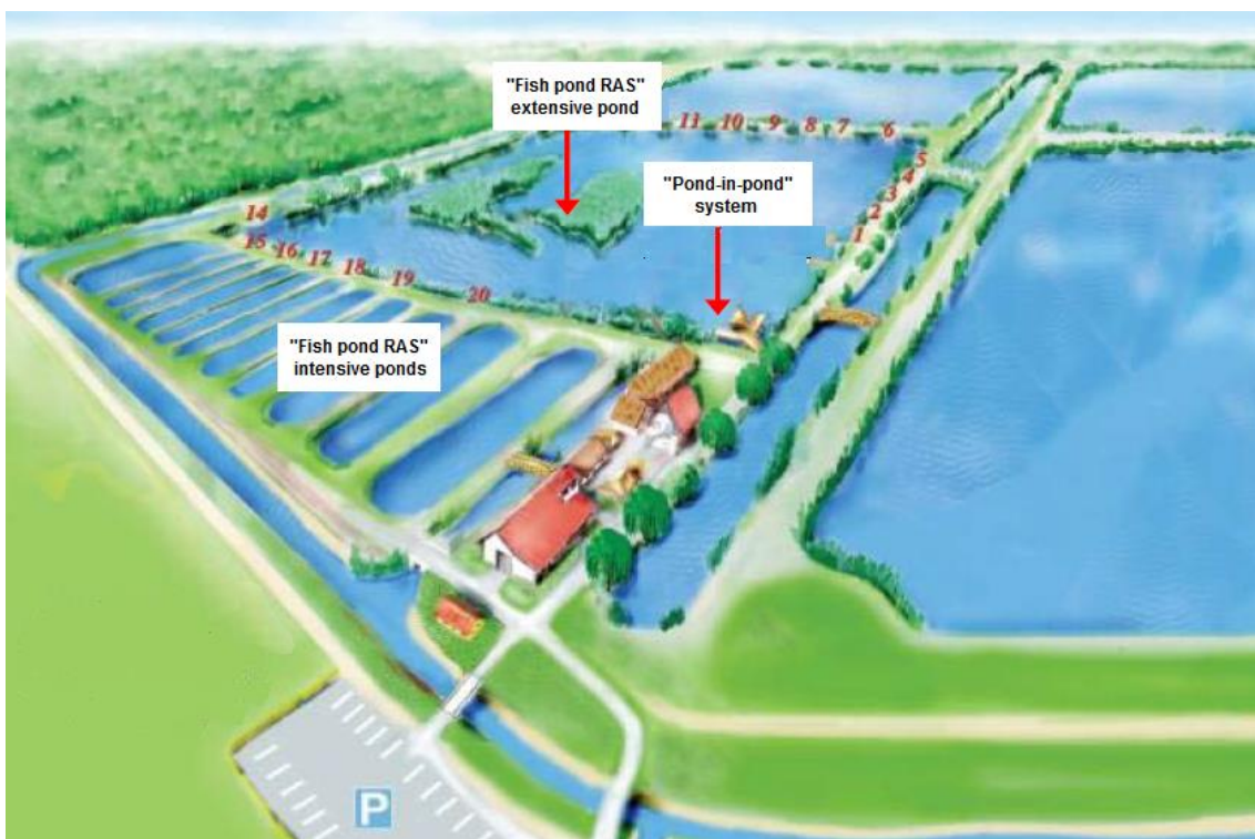
Figure 1 – "Pond-in-pond" and the "fish pond Recirculating Aquaculture System (RAS)" components in the fish farm of the "Jaszkeri "Halas" Kft"
